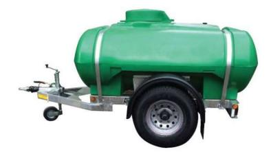
**CHASSIS:** Constructed from 5mm pressed steel section fully welded with a front standing plate and 100 x 50 RSC 'A' frame drawbar.
