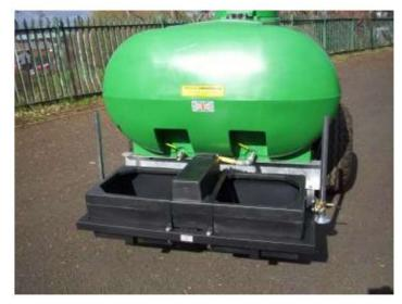
**CHASSIS** Constructed from 5mm pressed steel section fully welded with a 100 x 50 R.S.C 'A' frame drawbar and a front standplate.
