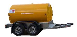
CHASSIS: Constructed from 100 x 50 RSC fully welded with front standing plate and an 'A' frame drawbar. Hot dip galvanised.
