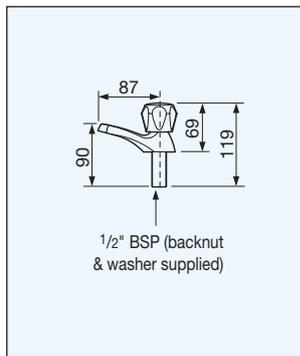
These taps are packed individually with both a red and blue bezel and are normally used in cold tap form to match the TXH01.
