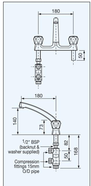
This is similar in operation to the vented hot tap but has the additional advantages of mixing the heated and cold water at the outlet and is ideally suited to kitchen use.
