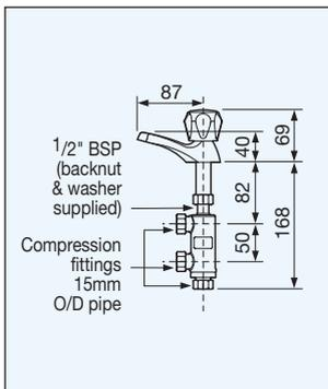
This tap is constructed to control the flow of incoming mains water supply to an open outlet type electric water heater. This displaces the heated water in an unrestricted flow through the tap's permanently open outlet. This vented hot tap is for full bore plumbing.
