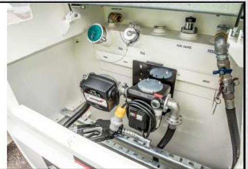
**YARDMAX-FM-240V:** Electric fuel pump for dispensing diesel. Pump fitted with bypass, 2m suction hose, mechanical flow meter, 4m delivery hose & auto nozzle for safe refuelling.
