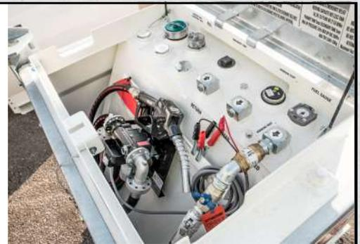
**YARDBAK-FM-12:** Electric fuel pump for dispensing diesel. Pump fitted with bypass, 2m suction hose, mechanical flow meter, 4m delivery hose & auto trigger nozzle for safe refuelling.
