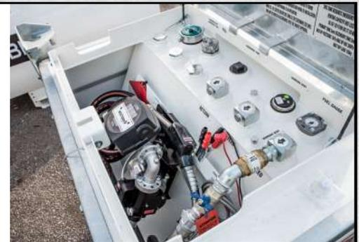
**FIELDPAK-FM-PE:** Petrol engine fuel pump for dispensing diesel. Pump fitted with bypass, 2m suction hose, mechanical flow meter, 4m delivery hose, nozzle holder & auto trigger nozzle for safe refuelling.
