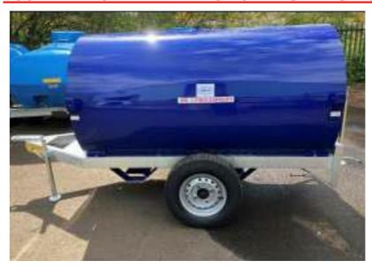
**CHASSIS:** Constructed from 100 x 50 RSC fully welded with front standing plate and 'A' frame drawbar. Hot dip galvanised.
