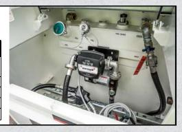
**YARDMAX-FM-110V:** Electric fuel pump for dispensing diesel. Pump fitted with bypass, 2m suction hose, mechanical flow meter, 4m delivery hose & auto nozzle for safe refuelling.
