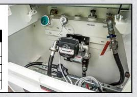
**YARDMAX-FM-24V:** Electric fuel pump for dispensing diesel. Pump fitted with bypass, 2m suction hose, mechanical flow meter, 4m delivery hose & auto nozzle for safe refuelling.
