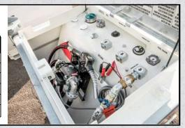
**YARDPAK-FM-12:** Electric fuel pump for dispensing diesel. Pump fitted with bypass, 2m suction hose, mechanical flow meter, 4m delivery hose & auto trigger nozzle for safe refuelling.
