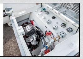
**FIELDPAK-FM-PE:** Petrol engine fuel pump for dispensing diesel. Pump fitted with bypass, 2m suction hose, mechanical flow meter, 4m delivery hose, nozzle holder & auto trigger nozzle for safe refuelling.
