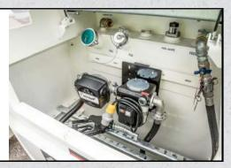
**YARDMAX-FM-240V:** Electric fuel pump for dispensing diesel. Pump fitted with bypass, 2m suction hose, mechanical flow meter, 4m delivery hose & auto nozzle for safe refuelling.
