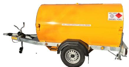
**COUPLING:** Knott-Avonride 2000kg posibrake over run auto reverse c/w spring assisted handbrake lever, breakaway cable & 40mm ring eye or 50mm ball. **ANCILLARY EQUIPMENT:** Moulded mudguards, mud flaps, rear support stand, telescopic front jockey wheel, Side reflectors, front reflectors, full road lighting c/w 13 pin plug and 7 pin adapter.
