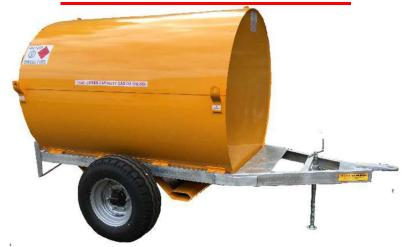
**CHASSIS:** Constructed from 100 x 50 RSC fully welded with front standing plate and 'A' frame drawbar, Hot dip galvanised.
