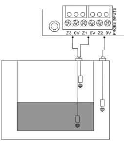
There are six probe connections, which are located as shown here. The probe wired to the 'High' connection is positioned topmost in the tank, and is used to alert that an overfill has occurred. Whereas the probe in the 'Low' connection should be placed near the bottom of the tank, to indicate a low level. The 'Bund'
