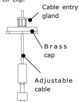
The position of the float can be adjusted to the required height by loosening the cable entry gland on the brass cap.
