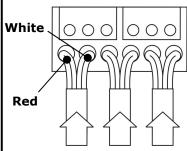
You will notice that in the probe cable there are two wires, one red and one white. The red wire should be connected to the Z(x) terminal and the white wire to the corresponding 0V terminal. The colour is actually irrelevant but it is suggested for simplicity all wires to the 0V' connections are kept the same. For Zone set-up see page 10.
