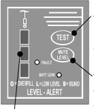
To test the alarm press and hold the 'test' button, whilst the button is pressed all the configured zones, fault, red lamp and sounder will activate. If no zones are active all lights and the sounder will stop when the button is released.
