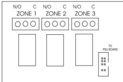
The relay outputs are optional and can be added to the unit at anytime. They allow switching to external equipment when either the High, Bund or Low alert is triggered. For example, a pump is activated in the event
