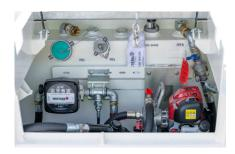
**FIELDMAX-FM-PE:** Petrol engine fuel pump for dispensing diesel. Pump fitted with bypass, 2m suction hose, mechanical flow meter, 4m delivery hose, nozzle holder & auto trigger nozzle for safe refuelling.
