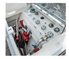
YARDPAK-12V/YARDPAK-FM-12V\*: Electric fuel pump for dispensing diesel. Pump fitted with bypass, 1.2m suction hose, mechanical flow meter\*, 4m delivery hose & auto trigger nozzle for safe refuelling.
