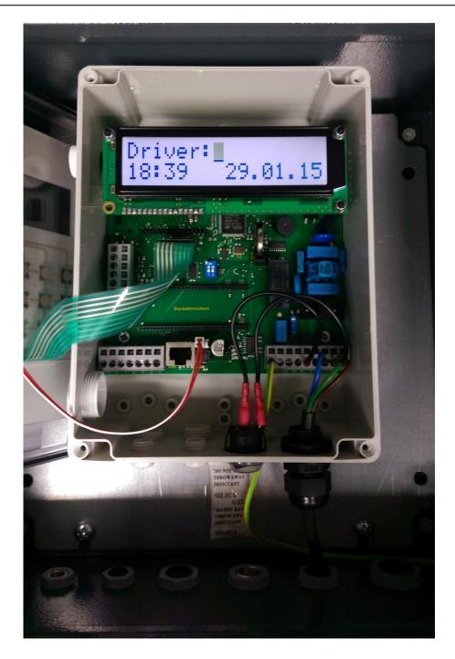
The HDA internals kept simple and straight forward. LAN and Wi-Fi capable.
