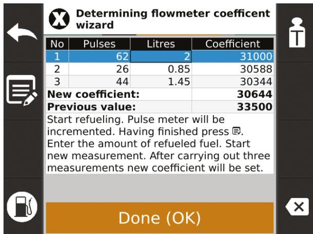
To save calculated value of the new ratio press **OK**. If you do not want to save it press **ESC** or **F1**. To save the changes exit flow meter calibration menu by pressing **ESC** or **F1** and confirm changing the coefficient by pressing **OK**.
