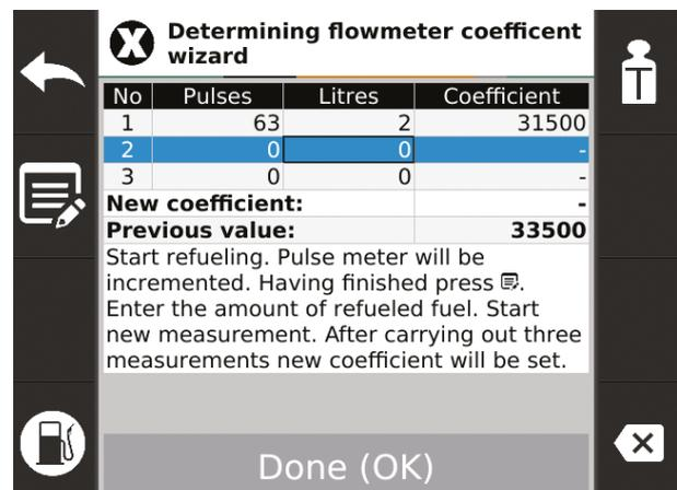
The line with current measurement is highlighted. When filling the flask with fuel the terminal counts pulses and displays them in "Pulses" column.
