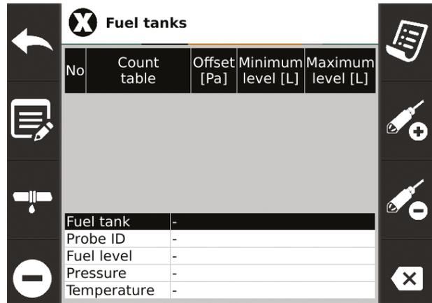
When you first start the terminal no fuel probes are visible. They must first be addressed. To address the probe connect it to the terminal.
