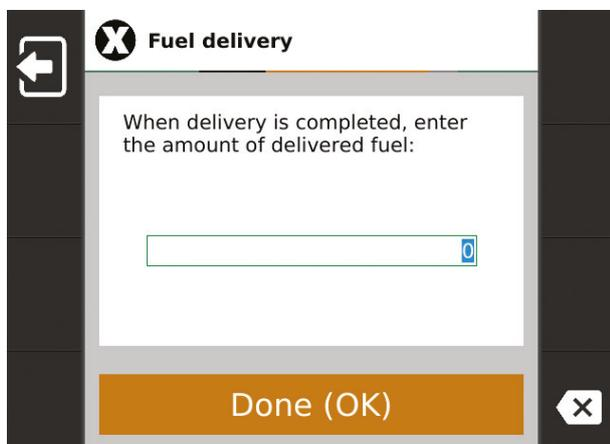
Start refueling. Having finished enter the amount of added fuel using the keyboard and press **OK**. The amount of fuel must be confirmed.
