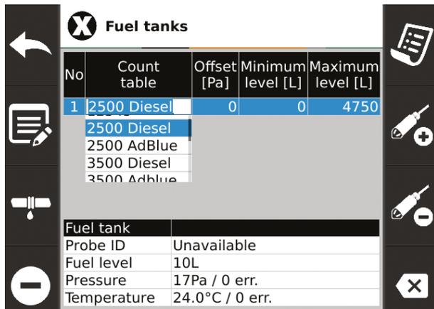
After pressing **F2** (field edit mode) select appropriate options depending on tank capacity by using **up/down arrows** (standard tables for the selected containers are saved) and type of fuel stored in it (diesel or ad-blue).
