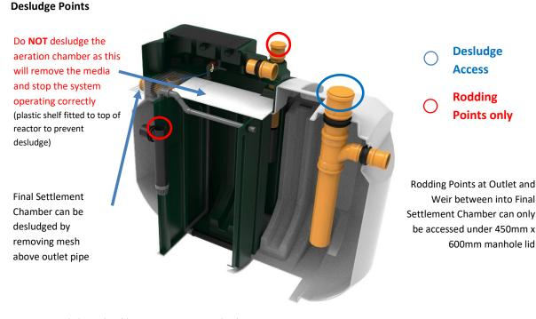
Figure 13: Desludge and Rodding Access points on HydroClear range
