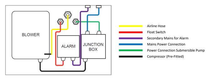
Figure 10: Connections inside External Air Blower Housing (Pumped Outlet Version)
