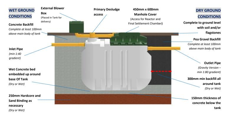
Figure 4: Typical Installation - Dry and Wet Ground Conditions (HC6 model)
