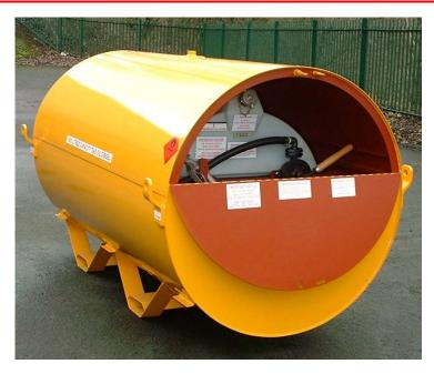
OUTER BUND TANK: Constructed from 3mm Mild Steel, cylindrical in section. Removable top section.4 lifting eyes on tank corners. Built-in fork truck sockets in base of tank. Stainless steel Hinged rear access door, fully lockable.
